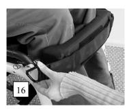
• Attach the two eyes of the knee support to the double-head screws on both sides of the wheelchair.
