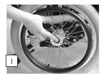
The **LEVO** *KID & JUNIOR* standard is fitted with pneumatic tyres. The diameter of the wheels depends on the seat height of the wheelchair. Thanks to the quick-release axles, the rear wheels can be easily removed and set back in place (see photo 1).
