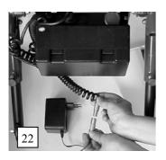
• To charge the batteries pull the hand control cable out of the armrest and connect the charger plug and the hand control cable. Then plug the charger itself into the mains (see photo 22).
