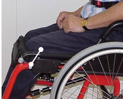
Knee support attachment screw beyond center of knee
